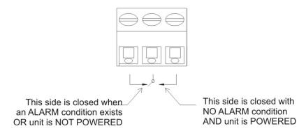
Figure 3-3: Contact ID for FAILSAFE Relay Operation
